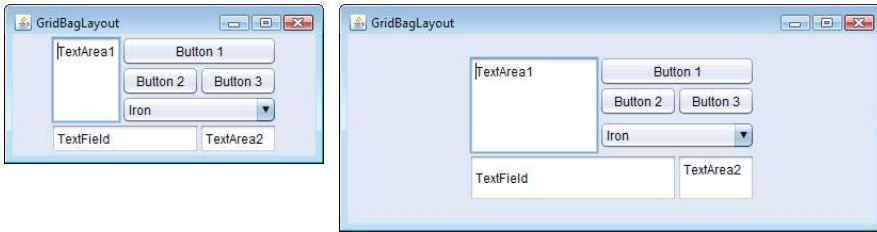
Fig. 22.20 | GridBagLayout with the weights set to zero.
